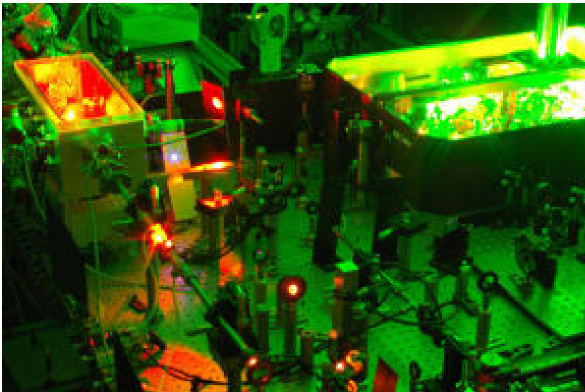
Laser system for generating ultra short x-ray pulses which is used in the experiment to make the recordings. (Credit: Rohwer et al., Copyright: CAU)
